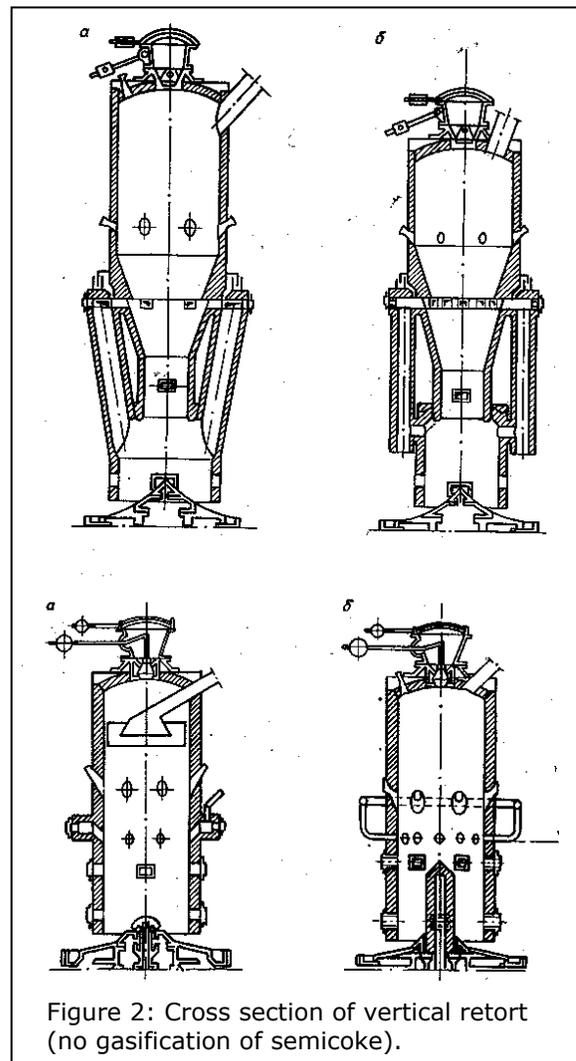
Figure 2: Cross section of vertical retort (no gasification of semicoke).
