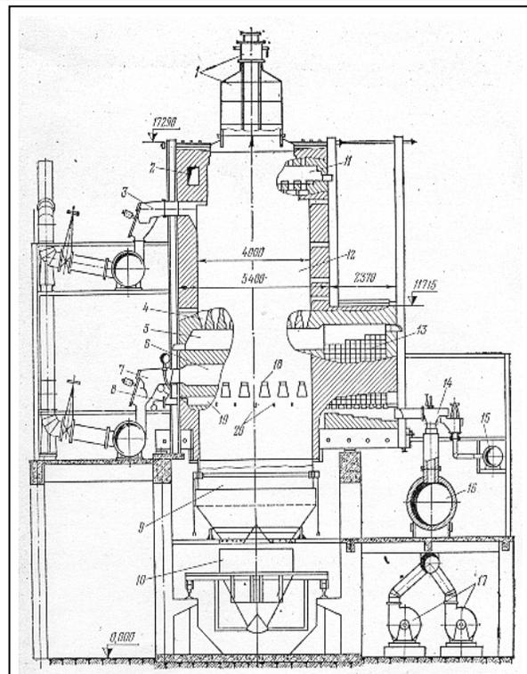
Figure 4: Cross section of the chamber oven
