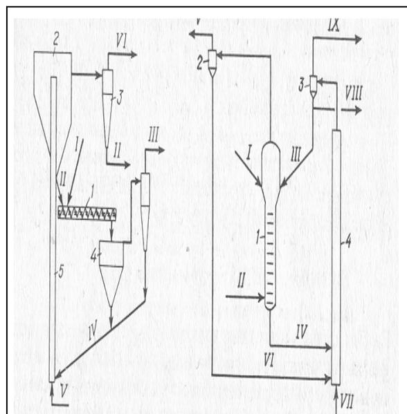
Figure 5: Flow diagrams of the Lurgi-Ruhrgas and Chevron STB processes
