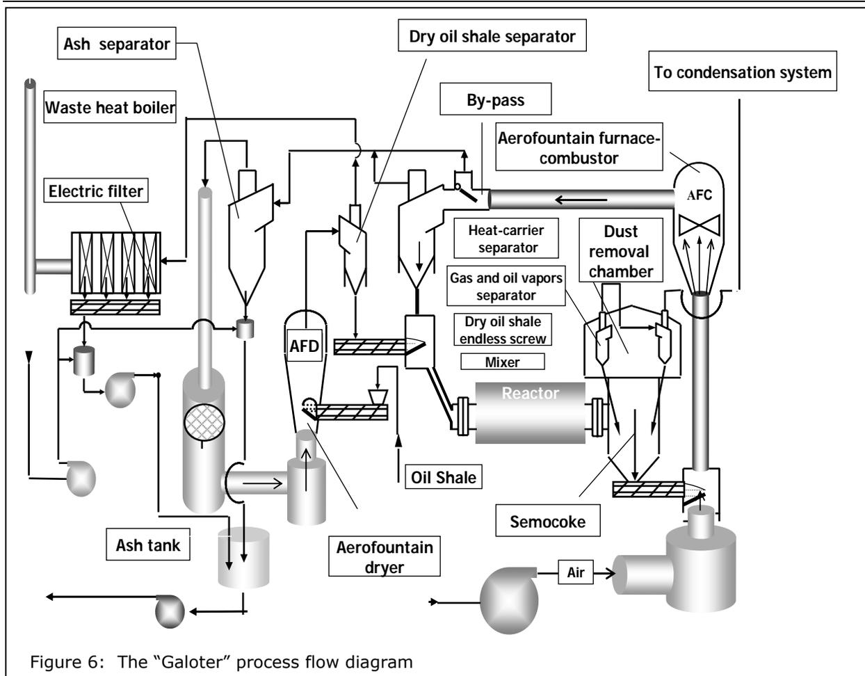
Figure 6: The "Galoter" process flow diagram
