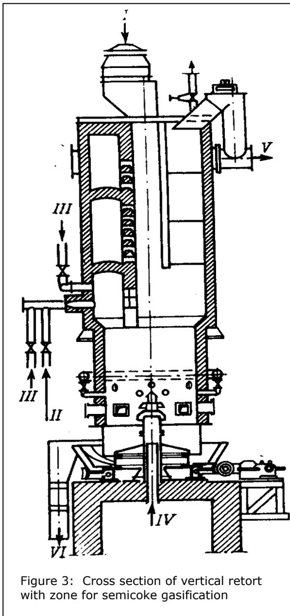
Figure 3: Cross section of vertical retort with zone for semicoke gasification
