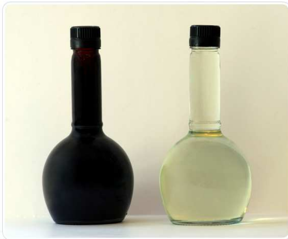
Before and After – raw shale oil and hydrotreated shale oil
