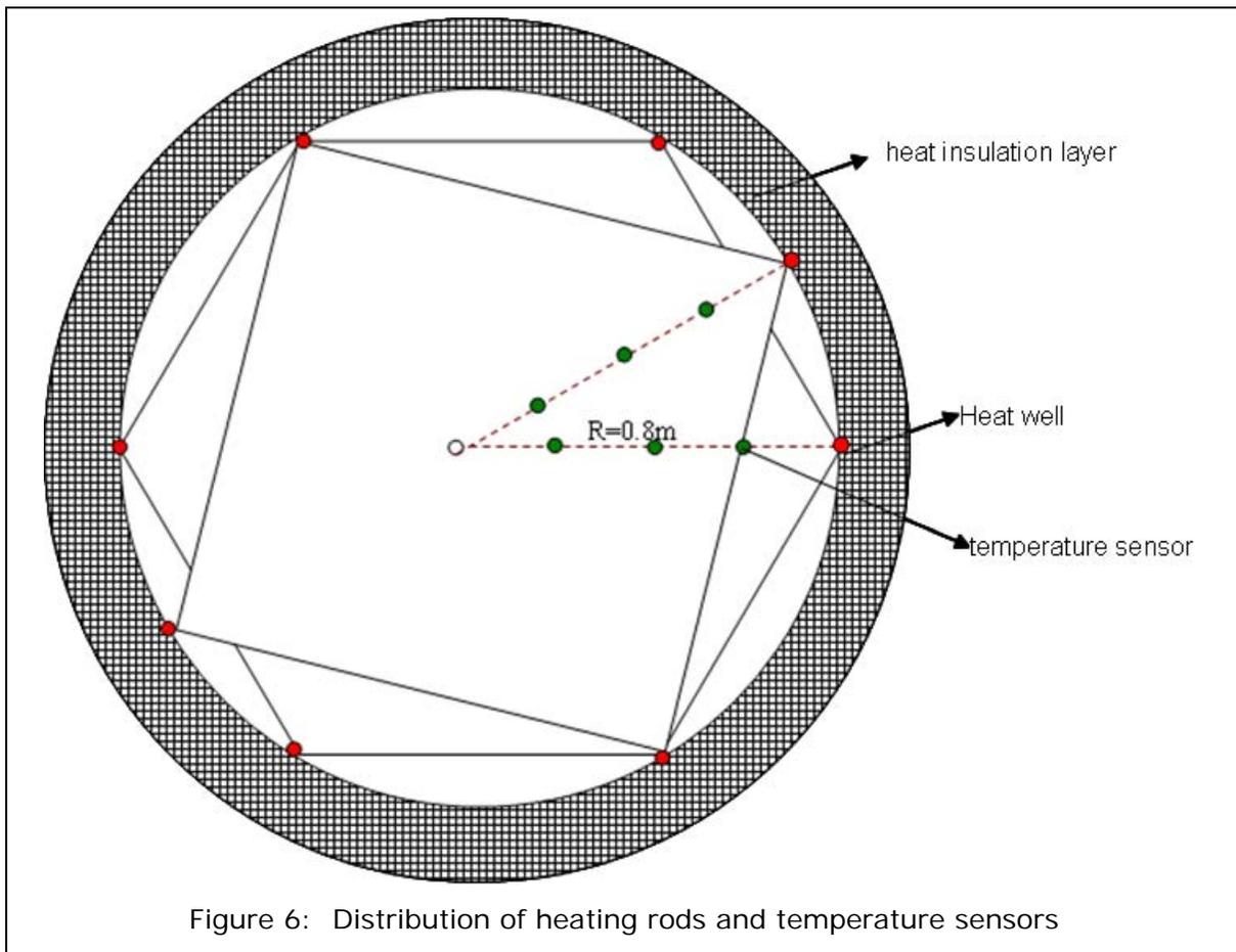
Figure 6: Distribution of heating rods and temperature sensors
