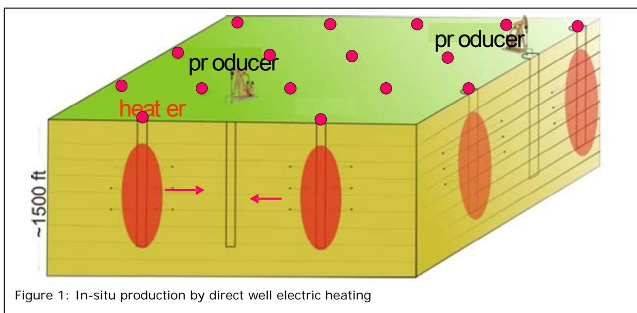
Figure 1: In-situ production by direct well electric heating
