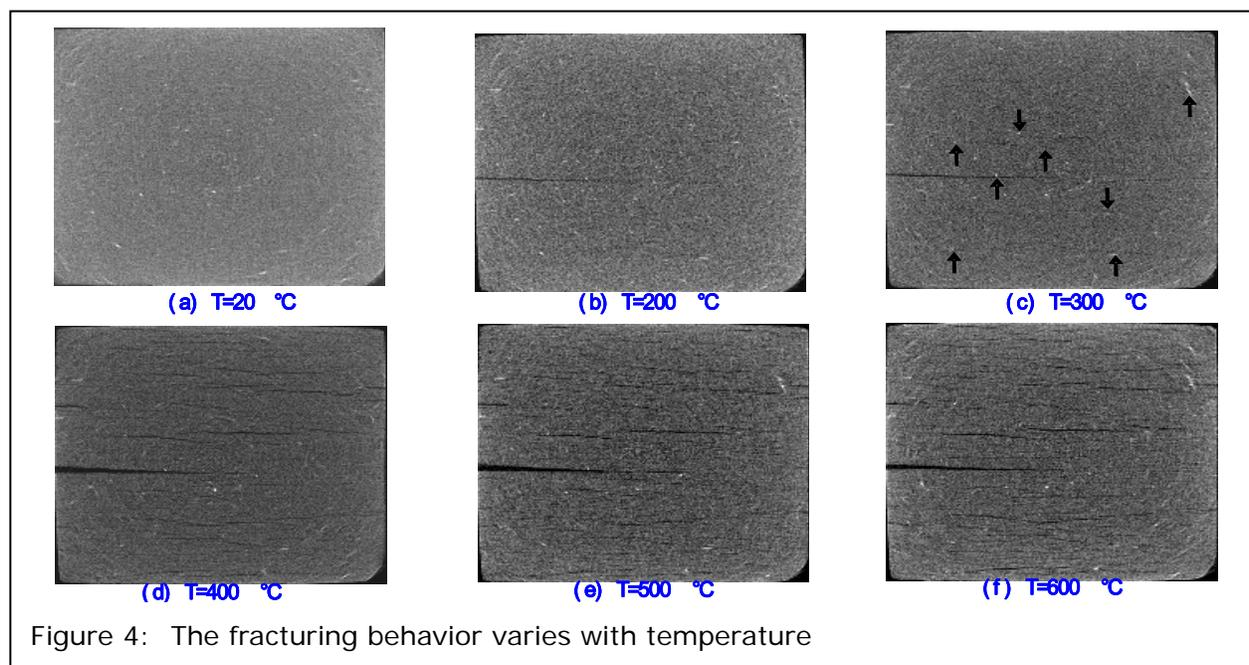
Figure 4: The fracturing behavior varies with temperature
