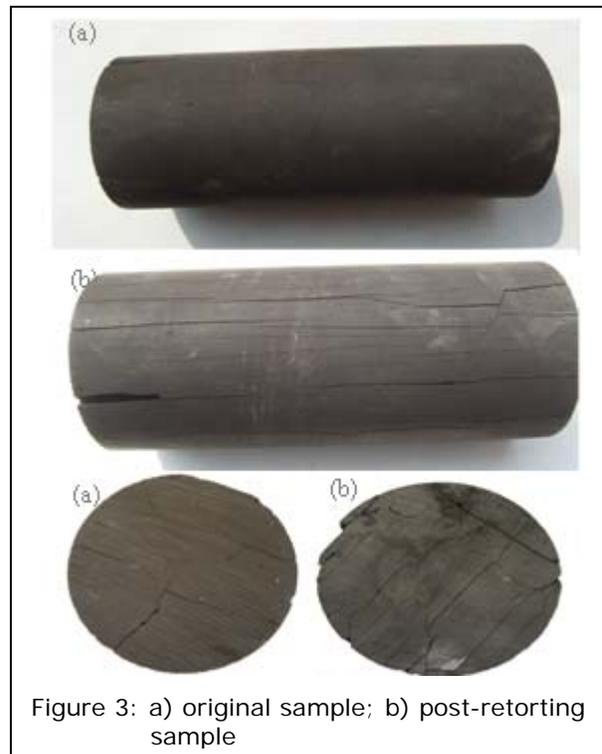
Figure 3: a) original sample; b) post-retorting sample
