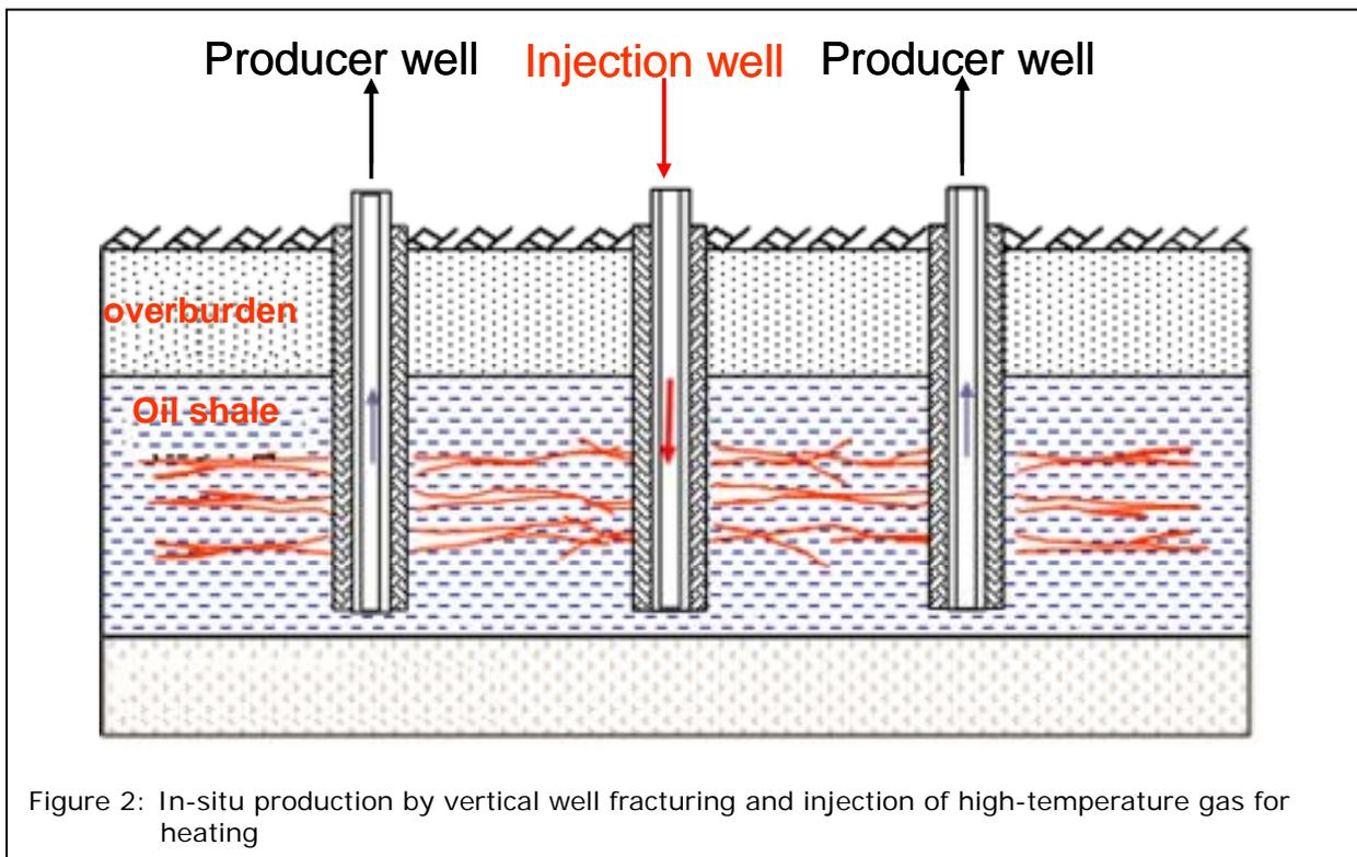
Figure 2: In-situ production by vertical well fracturing and injection of high-temperature gas for heating
