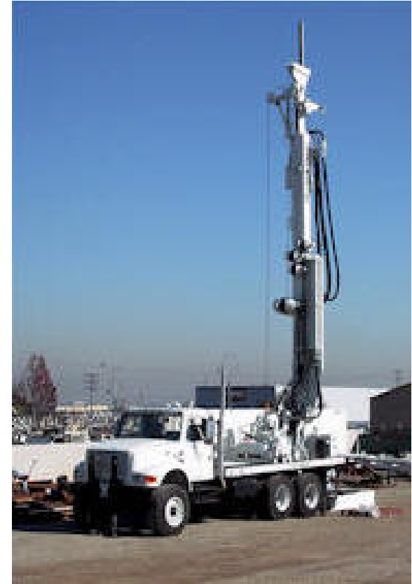
(Low cost truck mounted rig)
